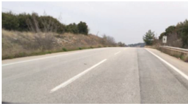
Figure 4: A combination of small radius vertical crest with horizontal curve.
