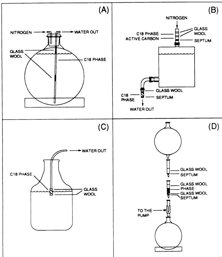
Figure 1. Four different all-glass extraction apparatuses (not in scale).
