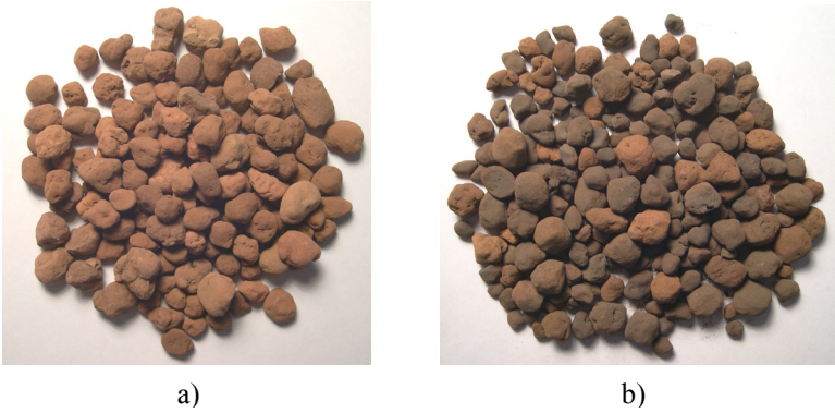
Figure 1: Sintered ash-derived aggregates a) LWA 1 and, b) LWA 2.
