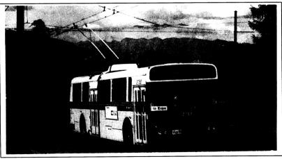
Points and crossings have been designed which offer the maximum dynamic reaction with the twin overhead collector heads mounted on the roof of the trolleybus, enabling them to be negotiated at higher service speeds than with the previous cast brass and iron designs. Route changing is done by electric solenoids commanded by switching circuits in the overhead or by radio signal from the vehicle.
