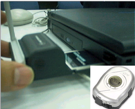
Figure 9: The system architecture of hardware -the connection of a PC, a wireless PCMCIA card, and a wireless GPS.
