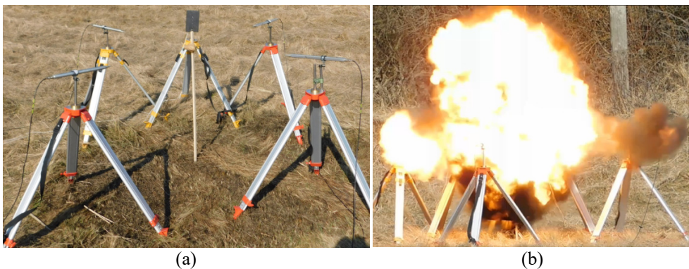
Figure 5: (a) Position of the instruments on the test site; and (b) and blast fireball after detonation.
