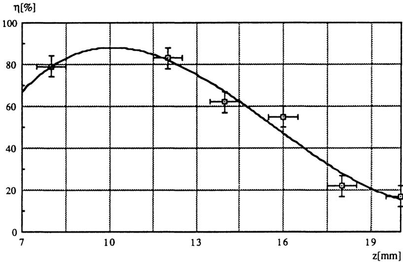
Fig. 3: Efficiency of powder deposition vs distance between nozzle and sample for Stellite.
