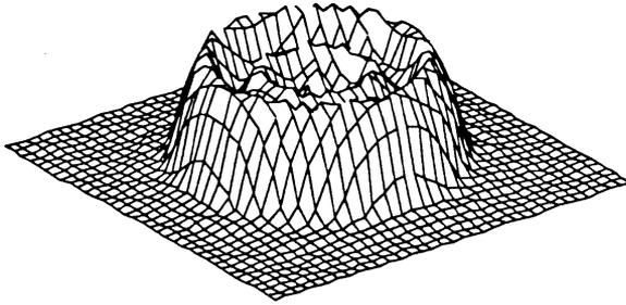
Fig. 4 : Intensity profile of the laser beam used in this work. Power range : 3 to 5 kW.
