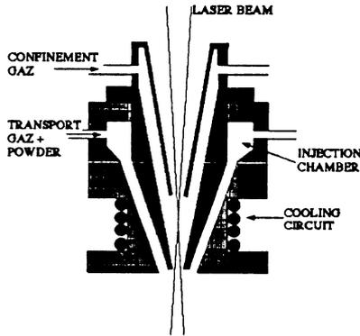
Fig. 1 : Sketch of a nozzle for coaxial distribution of powder and laser beam.
