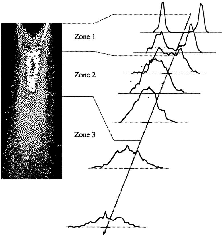
Fig. 5 : Density profile of the powder stream at different distances from the nozzle exit.
