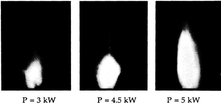
Fig. 8: Spatial development of the laser-induced plasma in the powder. Stellite blown with Argon.
