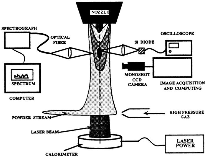
Fig. 6 : Experimental set-up used to study the interaction between the powder stream and the laser beam. Recorded signals are : laser radiation transmitted by the powder, temporal, spatial and spectral distribution of the photonic signals emitted by the heated powder.
