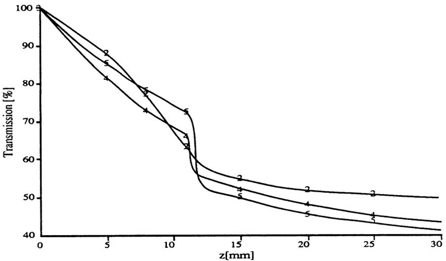
Fig. 7 : Transmission of the laser power by a stream of Stellite flown with Argon. Feeding rate : 30 g/mn. The 3 curves have been recorded for the following laser powers : 2 ->2 kW, 4 ->4 kW, 5 -> 5 kW.
