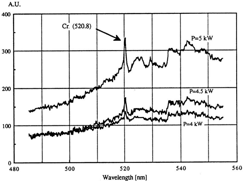
Fig. 9: Spectra of plasma induced in a stream of Stellite (Co 58%, Cr 30%, W 10 %, C 2%), recorded for three different laser powers. The spectra is recorded in the lower part of zone 2 defined on Fig. 5.
