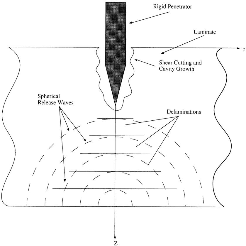
Figure. 1 A Schematic of the Delamination in a Composite Laminate Due to Penetration by a Metal Projectile [4]
