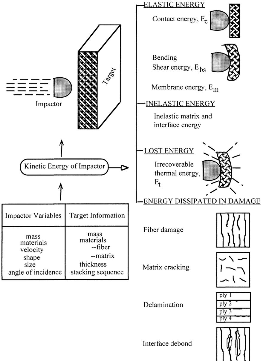
Figure 2 : Schematic of energy balance approach in high impact event
