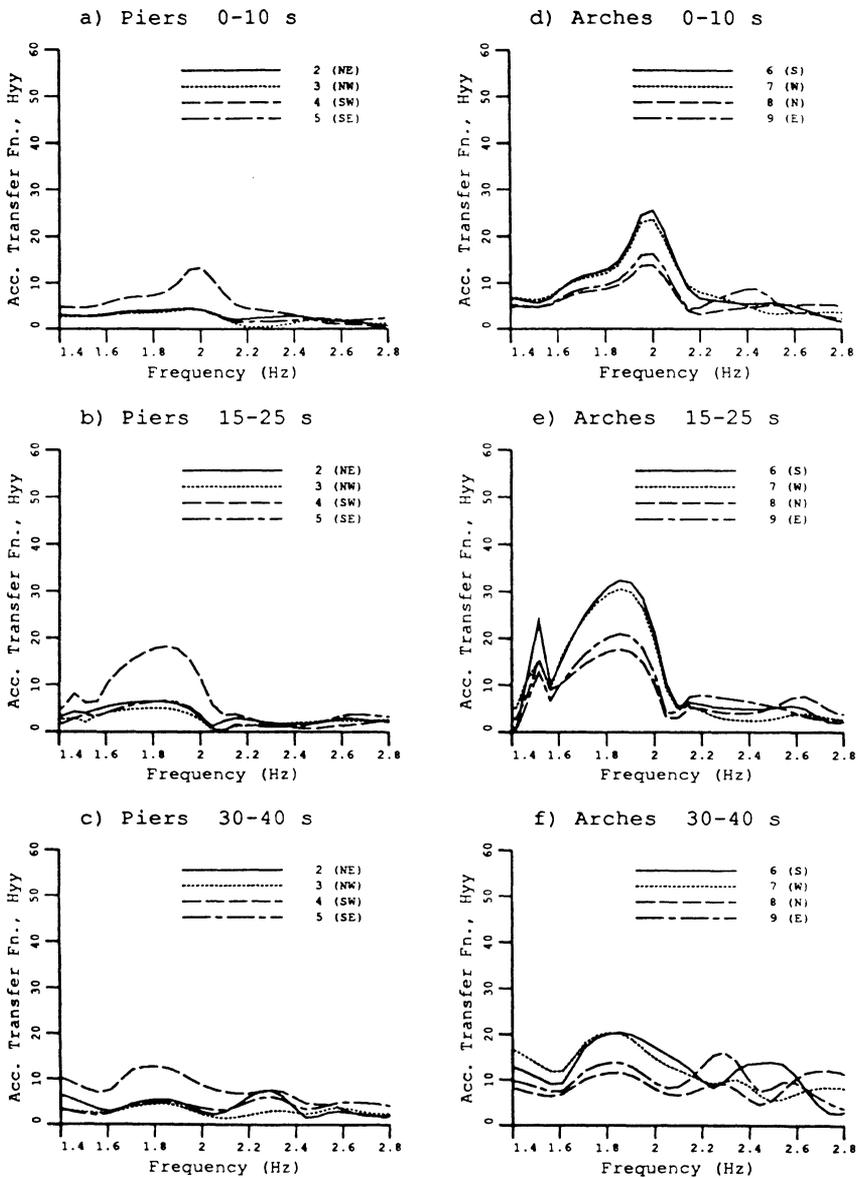
Figure 6. Transfer functions for N-S response to N-S base input.
