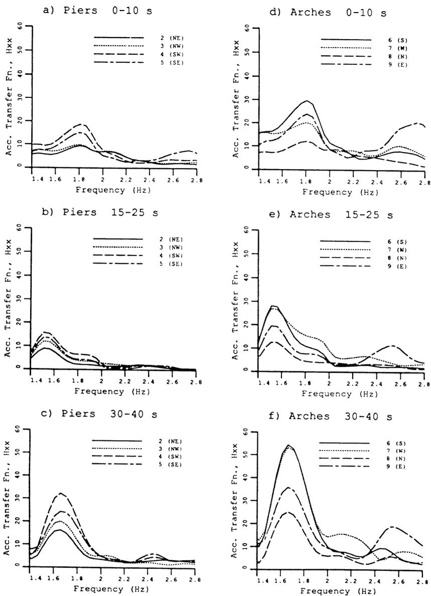
Figure 7. Transfer functions for E-W response to E-W base input.
