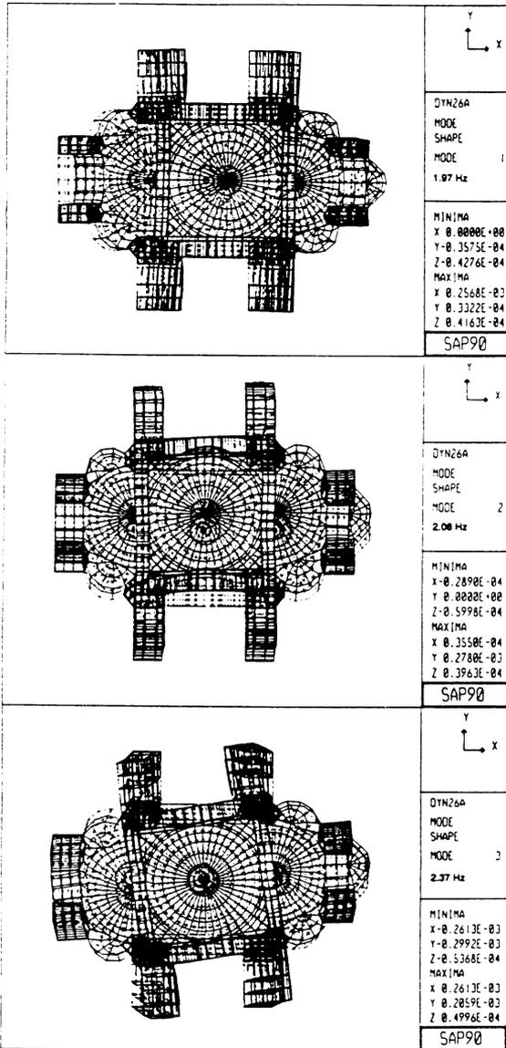
figure 1. Natural frequencies and mode shapes of primary structure model.
