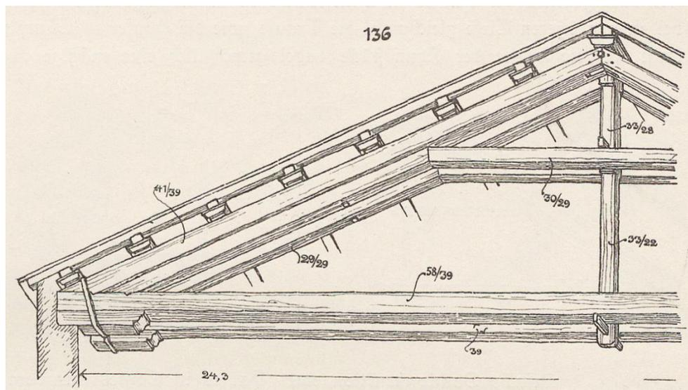
Figure 3: Ostendorf's illustration of the trusses of San Paolo FLM. (Source: Ostendorf, Figure 136.)
