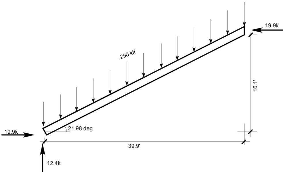
Figure 4: A diagram showing the analysis of the horizontal and vertical forces at the truss supports. Forces are shown in kips (1,000 pounds) or kips per lineal foot.
