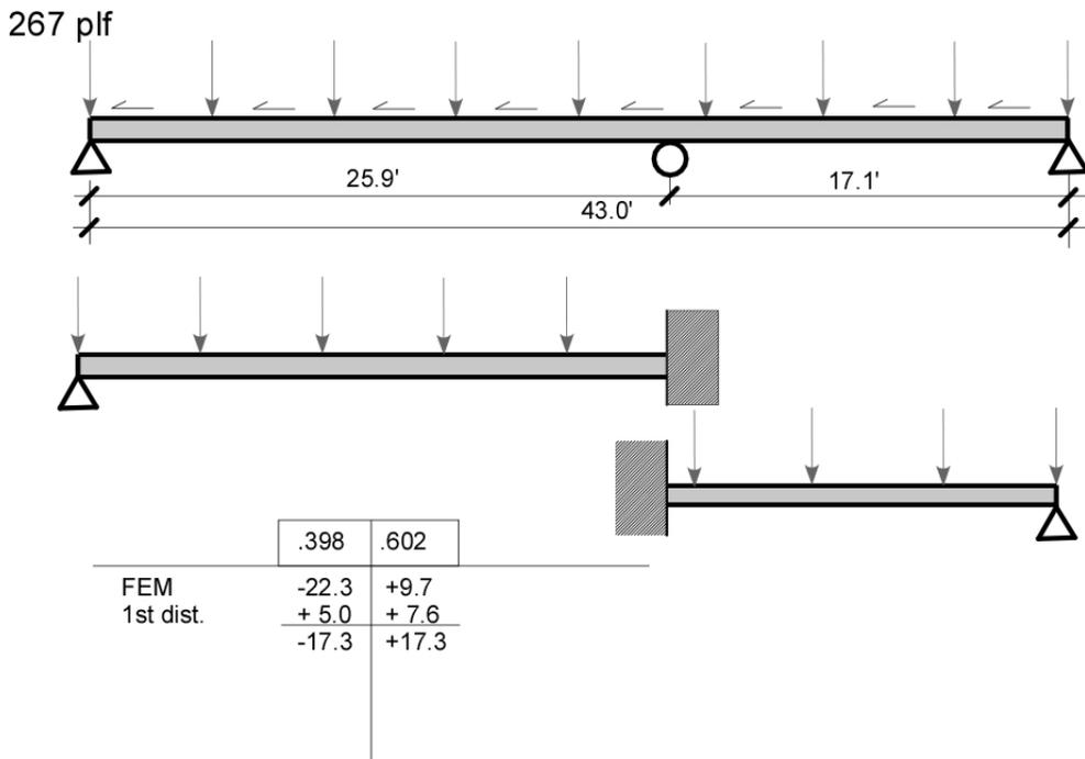
Figure 5: A diagram showing the moment distribution calculation of the moment in the upper chords at the point of intersection with the collar strut.
