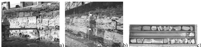
Figure 8: a,b: Coring at two different heights of the walls (450 and 1500mm) from the canal bed, c) one of the cores.
