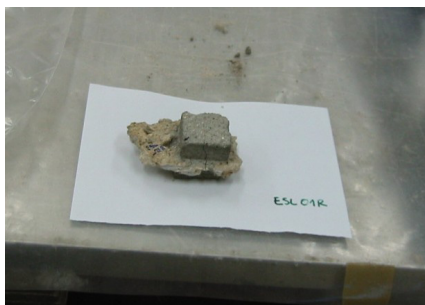
Figure 8: Samples from the Pisece Castle prepared for the compression test (render and joint mortar).
