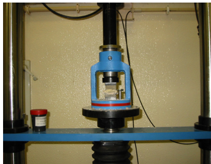
Figure 7: Compression test with confinement mortar.
