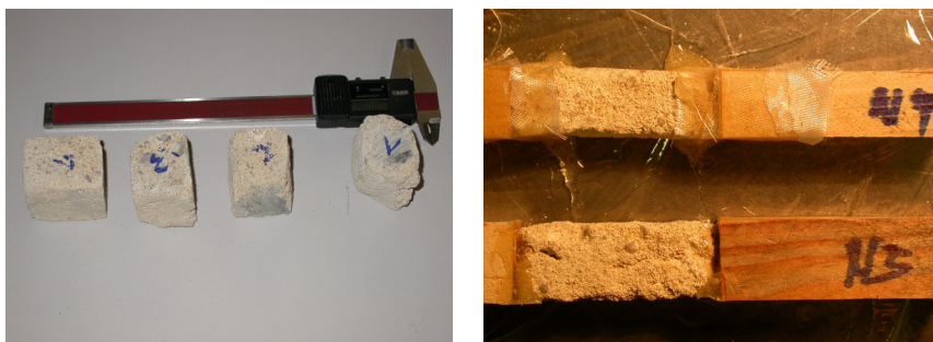
Figure 4: Mortar samples from one year old rubble wall cut to small ‘cubes’ and ‘prisms’
