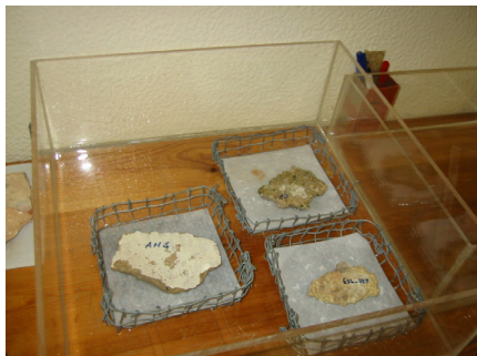
Figure 6: Capillarity test by the contact technique.
