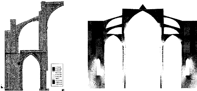
Fig. 3. Numerically predicted deformed shapes of the transverse sections of Tarazona (left) and Mallorca (right) cathedrals subject to gravity load (amplified by 100 ).
