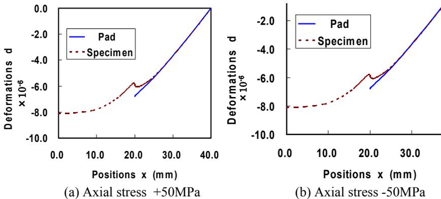
Figure 7: Calculated results of deformations on contact surfaces.
