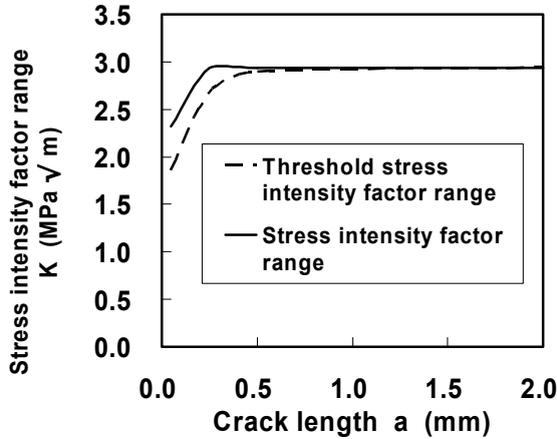
Figure 18: Comparison of operating stress intensity factor range with threshold stress intensity factor range. ( $\sigma_a=62\text{MPa}$ ,  $N=1.6\times 10^8$ , wear depth  $10\mu\text{m}$ ).
