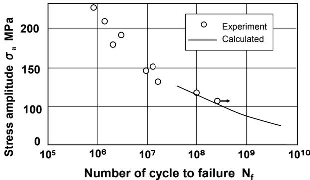
Figure 19: Estimated and experimental fretting fatigue S-N curves.
