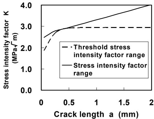
Figure 16: Comparison of operating stress intensity factor range with threshold stress intensity factor range. ( $\sigma_a = 140 \text{ MPa}$ ,  $N = 1 \times 10^7$ , without fretting wear).
