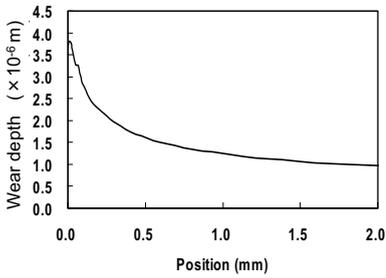
Figure 12: Calculated result of wear ( $\sigma_a=62\text{MPa}$ ,  $N=3.6\times 10^7$ ).
