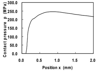
Figure 13: Calculated result of contact pressure. ( $\sigma_a=62\text{MPa}$ ,  $N=1.6\times 10^8$ ).
