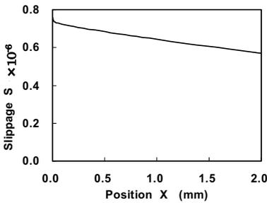
Figure 8: Calculated results of slippage in half loading cycle. (-50Mpa  $\blacktriangleright$  +50MPa).
