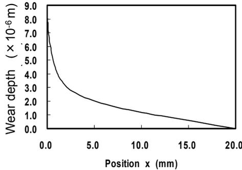
Figure 14: Calculated result of wear. ( $\sigma_a=62\text{MPa}$ ,  $N=1.6\times 10^8$ ).
