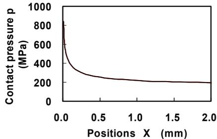
Figure 9: Calculated result of contact pressure distributions near contact edge.
