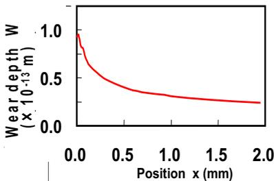
Figure 10: Calculated result of wear in loading cycle. (-50Mpa  $\blacktriangleright$  +50Mpa).
