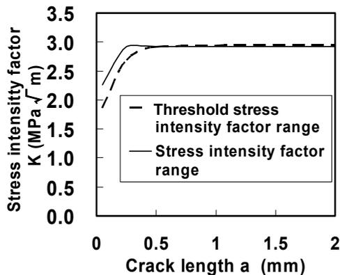
Figure 17: Comparison of operating stress intensity factor range with threshold stress intensity factor range. ( $\sigma_a = 110 \text{ MPa}$ ,  $N = 2 \times 10^7$ , wear depth  $4 \mu\text{m}$ ).
