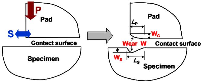
Figure 4: Wear analysis using contact pressure and slippage.
