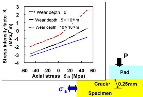
Figure 15: Calculated result of stress intensity factor for each wear depth.
