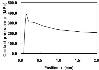
Figure 11: Calculated result of half contact pressure. ( $\sigma_a=62\text{Mpa}$ ,  $N=3.6\times 10^7$ ).
