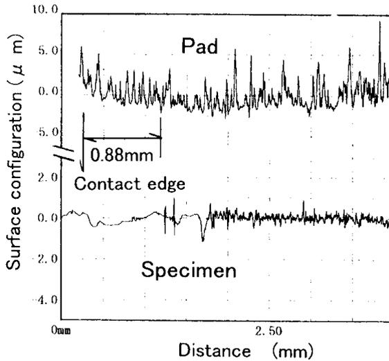
Figure 6: Experimental results of fretting wear. ( $\sigma_a=110\text{Mpa}$ ,  $N=2 \times 10^7$ , Ni-Mo-V Steel).
