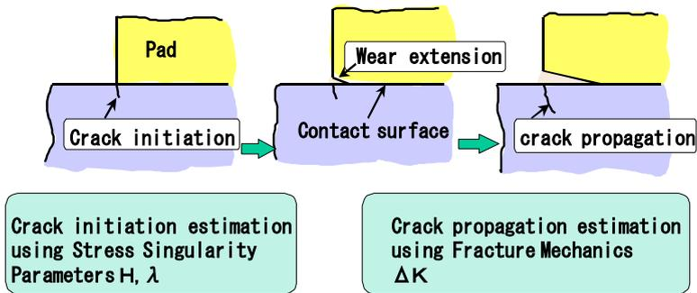
Figure 2: Fretting fatigue mechanisms in various processes.
