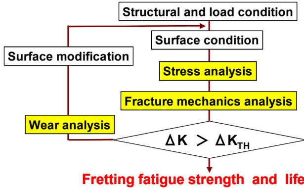
Figure 3: Flow chart of fretting fatigue life analysis.
