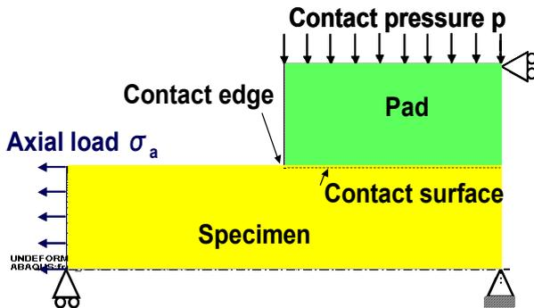
Figure 5: Fretting model for stress and deformation analyses.
