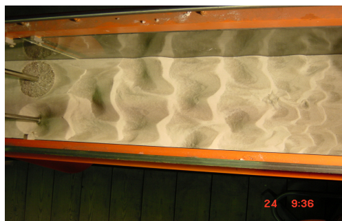
Figure 8: Picture obtained after an experiment with two circular cross-section piers, one of them with protection (destructive test).
