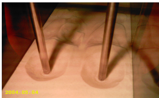
Figure 5: Picture from an experiment with a double circular cross-section pier.
