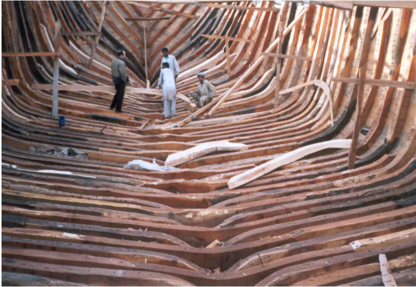
Figure 2: Interior section of a wooden dhow.
