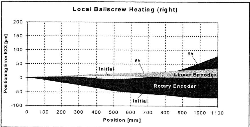
Figure 6: Positioning error – drilling cycle on the right table
