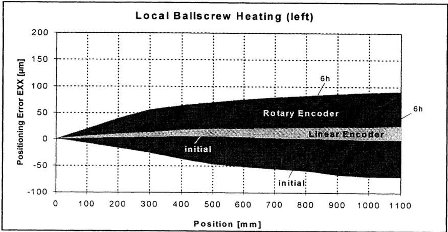
Figure 5: Positioning error – drilling cycle on the left table
