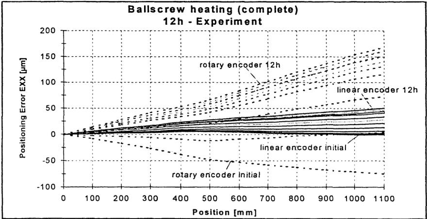
Figure 3: Positioning error, 12 hours full length traverse motion
