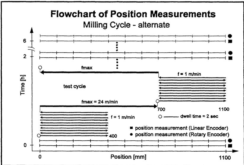
Figure 4: Test procedure
