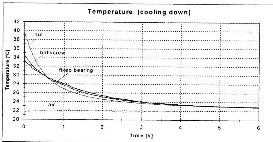
Figure 9: Cooling down phase
