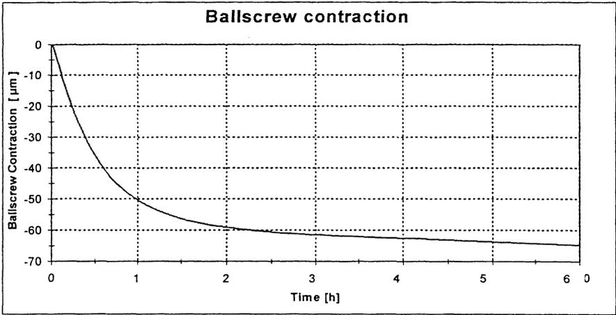
Figure 10: Cooling down, ballscrew contraction
