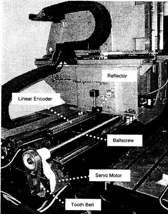
Figure 2: Drive components and position measurement systems
