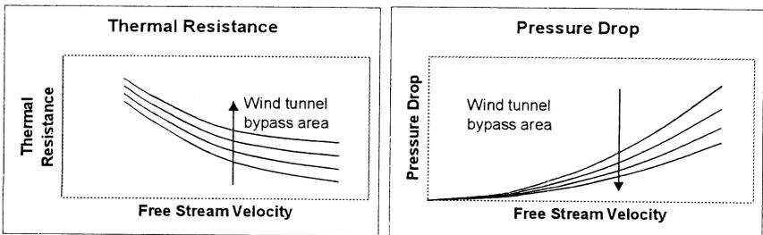
Figure 1. Effects of Bypass in Wind Tunnels
