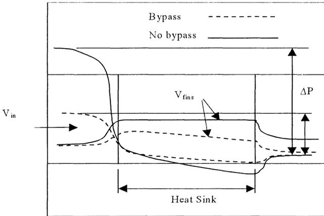
Figure 2. Pressure and Velocity Through Heat Sinks
