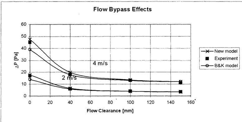
Figure 4. Comparison for Bypass Flow Pressure Drop
