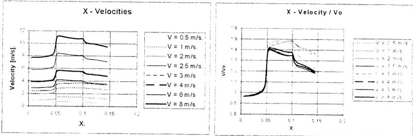
Figure 5: Longitudinal and Normalized Velocity through Heat Sink
