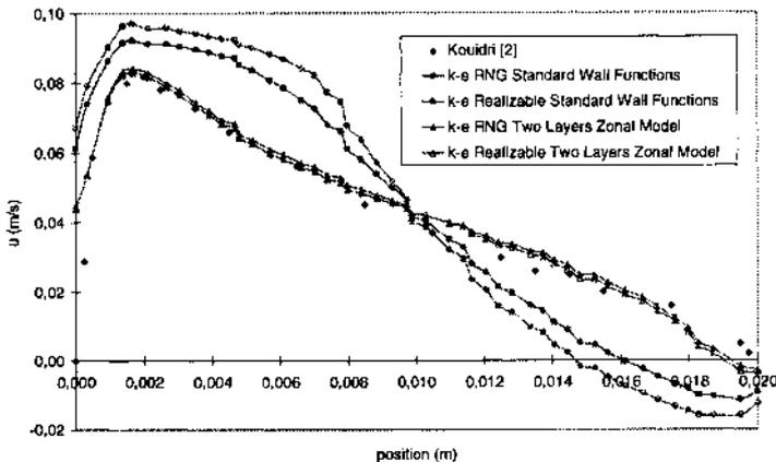
Figure 8: Velocity profiles at location A for  $Re = 1696$ .
