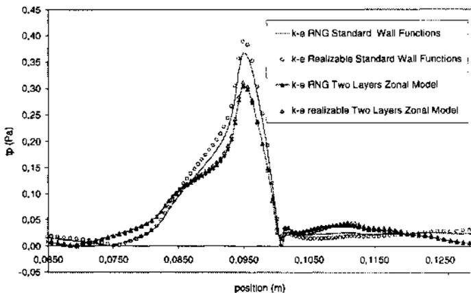
Figure 10: Wall shear stress profile at the top wall along one corrugation ( $Re = 1696$ ).
