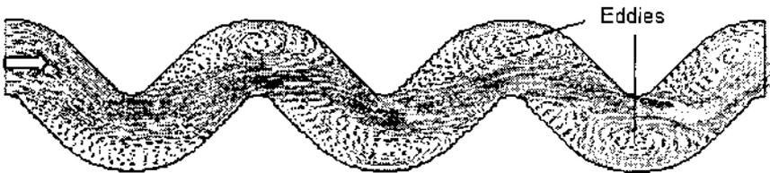
Figure 11: Velocity vector with LES model for  $Re = 8280$ .
