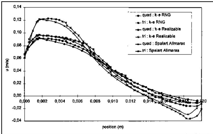
Figure 5: Comparison of results obtained with the two meshes ( $Re = 1696$ ) with standard wall functions.
