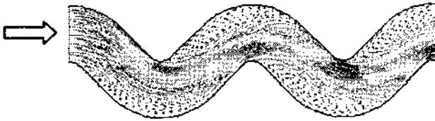
Figure 7: Velocity vectors with RNG ( $k, \epsilon$ ) model for  $Re = 1696$ .
