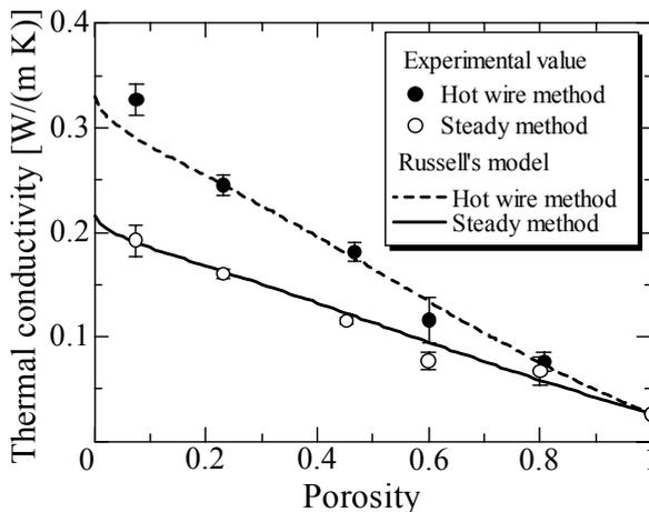
Figure 5: Effect of the porosity on the thermal conductivity.
