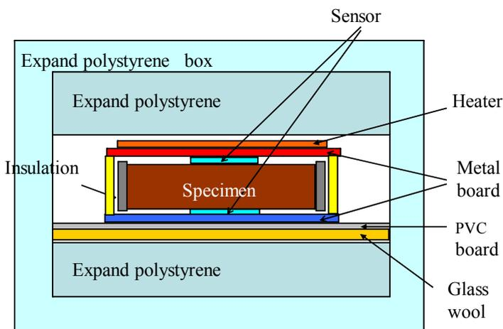
Figure 1: Schematic diagram of the steady state method.
