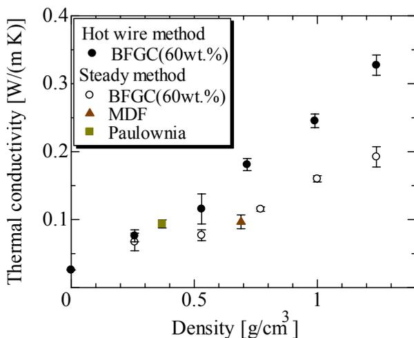
Figure 3: Relation between thermal conductivity and density and comparison of BFGC and other wood material.
