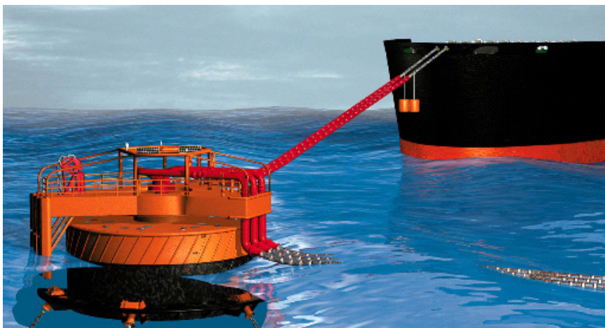
Figure 1: Offloading from a deepwater offloading buoy.
