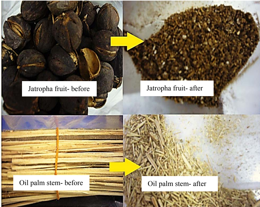
Figure 8: Jatropha fruits (upper) and oil palm stems (bottom), before and after undergoing grinding at medium speed of 25–30Hz.
