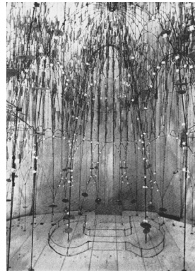
Figure 16: Chain shaped model of the church structure [6,7].
