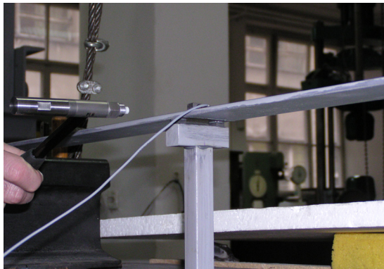
Figure 3: Incitement of the bridge model with hammer.
