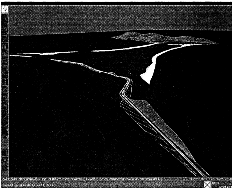
Figure 9: Road design combined with surface triangulation model of surrounding topography.
