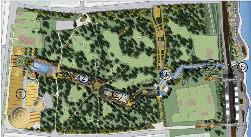
Figure 6: Master plan of the Star Grove Park. 1) Sport Palace. 2) Sport ground. 3) Building-bridge, 4) Anti-landslide frame, 5) Angara River embankment.
