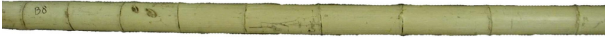
Figure 8: Increasing length of the internodes along the culm from the bottom part upwards.
