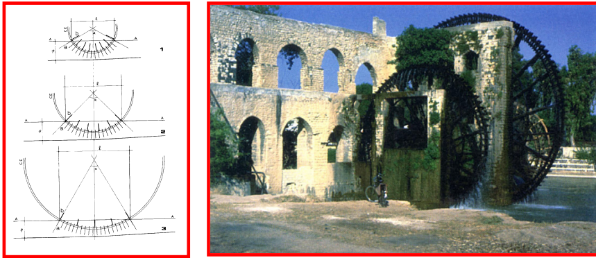
Figure 10: Scheme showing that, in proportion, the submerged areas tend to decrease in large wheels and to increase in small wheels (left). The group called “The four noria-s ”(right) at Hāma (Syria).
