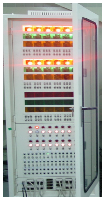
Figure 5: Track-side I/O emulation module.
