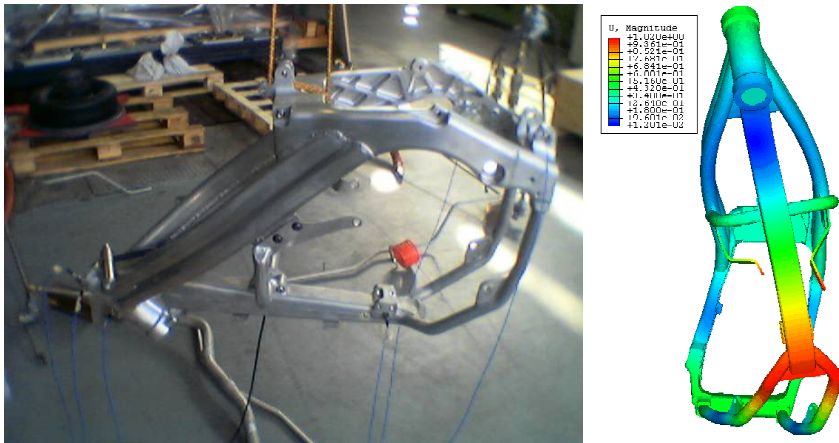
Figure 7: suspended frame for modal test, numerical vibration mode (230 Hz).
