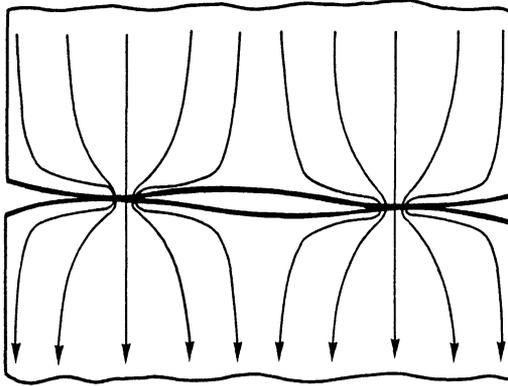
Figure 1: Current constriction to conducting spots in a contact surface.
