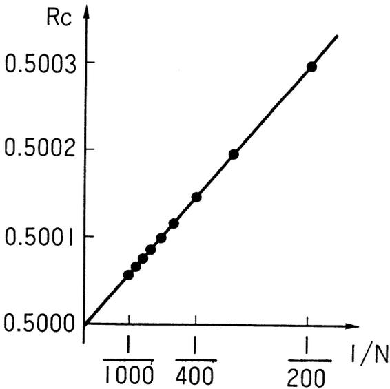
Figure 6: Estimation of constriction resistance  $R_c$  of circular spot when  $N \rightarrow \infty$ .
