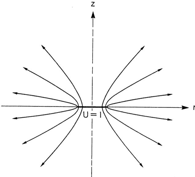
Figure 3: Steady current field for BEM.
