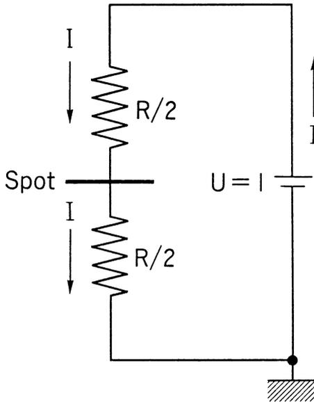
Figure 4: Equivalent circuit of Figure 2.
