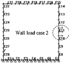
Unit traction is applied in the X-direction which is the direction of the first degree of freedom at the connection between the wall and the frame.
