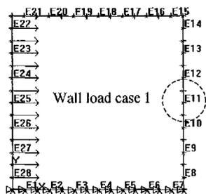
The element that demonstrates the connection between the wall and the frame. The length of this element is 0.4 m which is the same as the frame depth.
