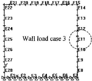
Unit traction is applied in the Y-direction which is the direction of the second degree of freedom at the connection between the wall and the frame.
