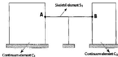
Fig. 1: A coupled skeletal frame with two continuum elements
