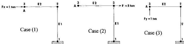
Fig. 12: The frame load cases.
