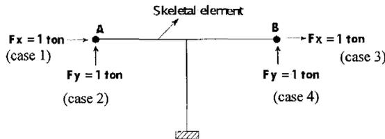
Fig. 6: The skeletal element  $S_1$  load cases.
