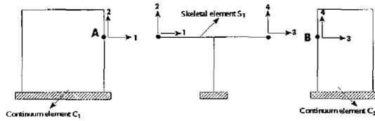
Fig. 3: The proposed sub-structures.
