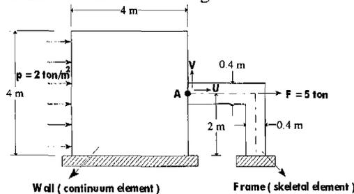
Fig. 7: Coupled wall-frame structure.
