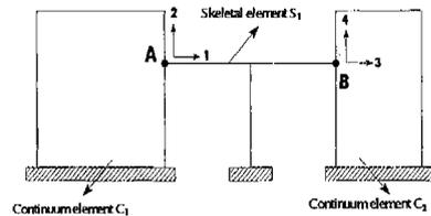
Fig. 2: The proposed degrees of freedom at the Connections points
