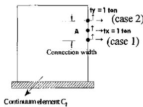
Fig. 4: The element  $C_1$  load cases.
