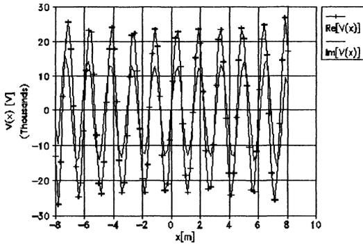
**Figure 3: Scattered voltage along the line**
