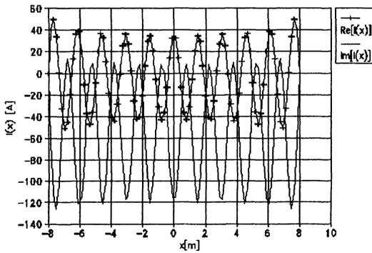
**Figure 2: Induced current distribution along the line**
