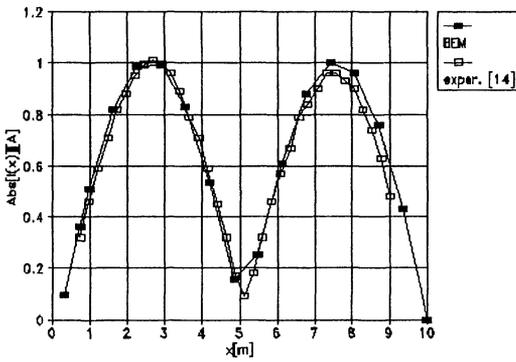
**Figure 1: Magnitudes of normalized current distribution along horizontal wire above lake water with:  $L=\lambda$ ,  $h/\lambda=0.00775$ ,  $a/\lambda=0.0015$ ,  $\epsilon_r=82$  and  $\sigma=0.092\text{S/m}$**
