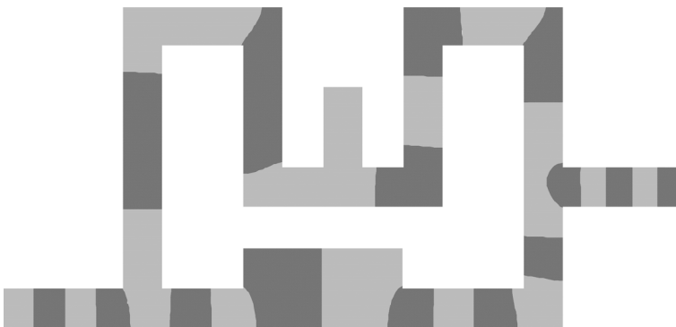
Figure 6: Potential distribution inside the conducting path of fig. 5, the potential difference between two equipotential lines is 0.1 V and the space between the two lines is coloured alternately.
