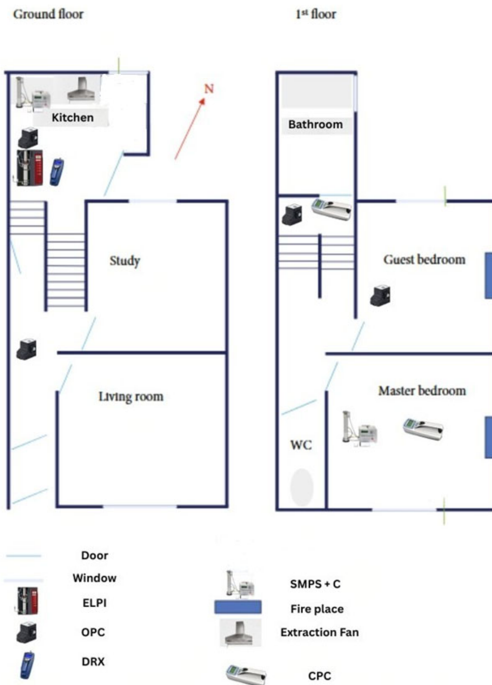
Figure 1: Layout of the two-storey SPHERE House showing instrument deployment for the experiments performed on 27 February 2025. The instrumental deployment for the experiments performed on 20 and 21 July 2016 can be found in Matthews et al. [21].
