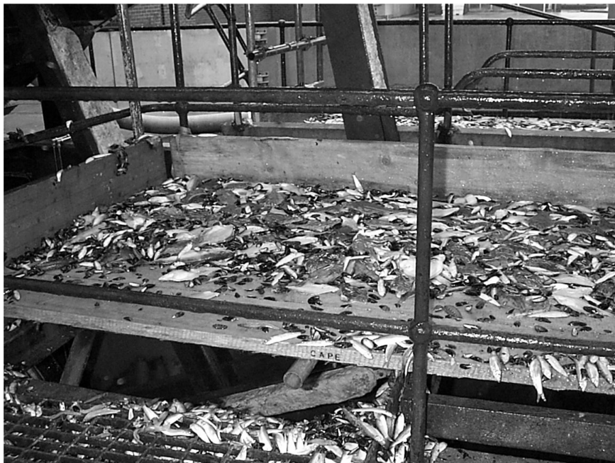
Figure 4: Fish collecting on temporary scaffold boards installed inside an operating drum-screen. The fish seen here have emptied from the buckets only after passing the collection hopper and would normally have fallen back into the screenwell and been recycled through the screening system.
