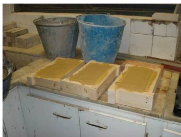
Figure 13: Lime mortar samples.
