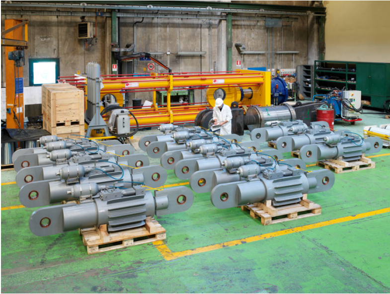
Figure 7: The fluid viscous dampers for the St. Francis Shangri-La Towers in Manila, Philippines.
