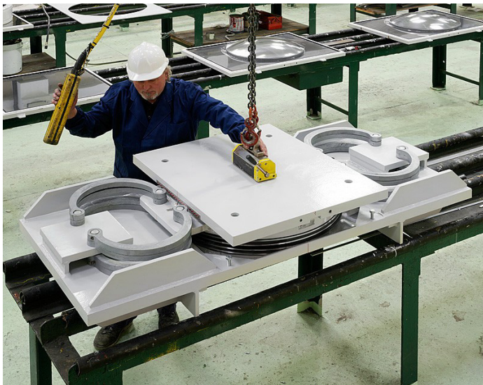
Figure 4: A flat surface slider with steel hysteretic dampers for the Madonna delle Lacrime” sanctuary in Syracuse, Italy.
