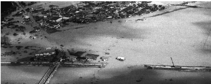
Figure 4.34: A part of levee collapse.
