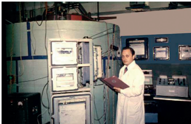
Figure 24: Ultrasensitive fast-acting differential microcalorimeter ( 10^{-8} W), containing spiral anisotropic thermoelements, using the Thomson transversal thermo-EMF (1986) [43].
