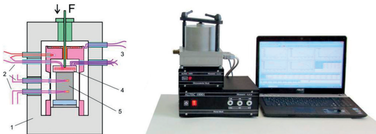
Figure 14: Schematic and appearance of the automated measuring setup for the material thermoelectric properties determination. 1 – thermostat, 2 – thermocouples, 3 – current leads, 4 – reference heater, 5 – sample.
