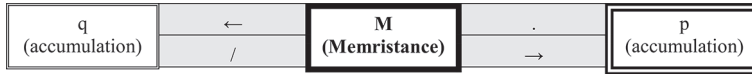
Figure 8: Direct relation between accumulation of effort and accumulation of flow: an accumulation of effort q divided by a memristance M gives an accumulation of flow p , and an accumulation of flow p multiplied by a memristance M gives an accumulation of effort q .
