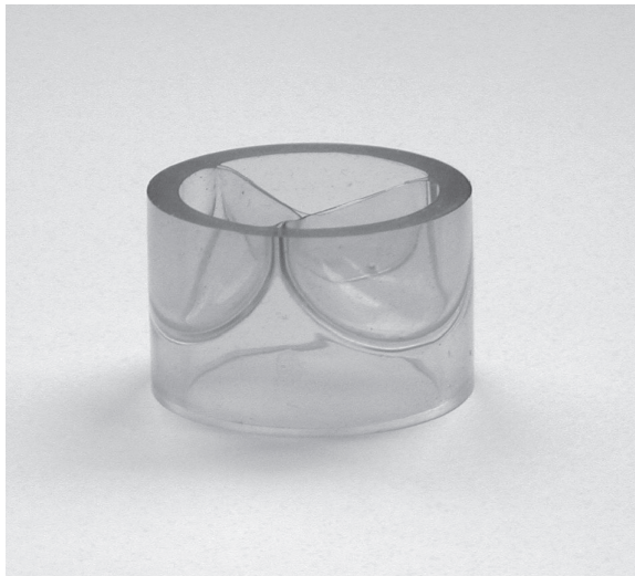
Figure 9: Trileaflet heart valve prosthesis made of polyurethane. The geometry of the valve duct is designed without valve sinuses [courtesy E. Hennig, Berlin].
