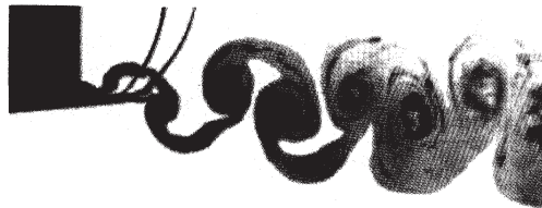
A Amplitude s_o = 5.0\text{mm} , f_{OS} = 2.50\text{ Hz} , v_\infty = 0.20\text{ m/s} , f = 10.72 , (2a/R) = 0.2274 , H_{mT} = -3.499\text{ N} , P_{mT} = 0.02668\text{ W} , Str_{\Lambda,m} = 0.0933
