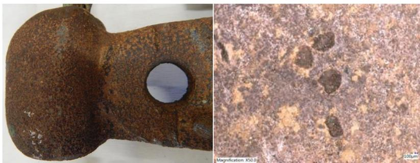
Figure 1: Surface of cast iron after 50 years of exposure – graphite particles.
