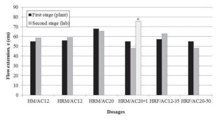
Figure 2: Slump flow obtained in the different dosages.
