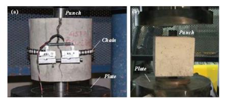
Figure 1: BCN test (A) on the cylindrical test specimen and with a strain gauge chain and (B) on the cubic test specimen and with control of the vertical displacement of the piston (without chain).
