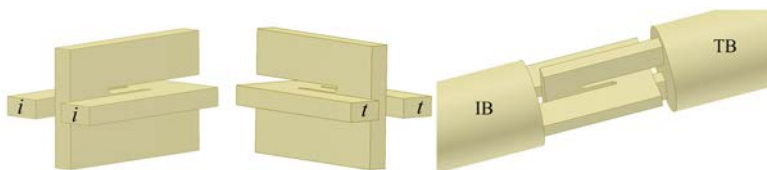
Figure 1: Type I compression-to-tension (CTC) structure. i represents the contact surface to the incident bar (IB) and t denotes that to the transmitted bar (TB).
