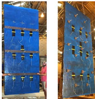
Figure 1: Finished strap anchorage retrofit (FT1 – left) and finished plate anchorage retrofit (FT2 – right).
