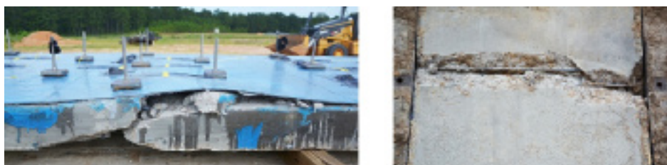
Figure 8: Intermediate crack-induced debonding (left) and concrete crushing (right) in the FT2 field test specimen.
