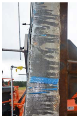
Figure 7: Concrete failure and debonding in FT1.
