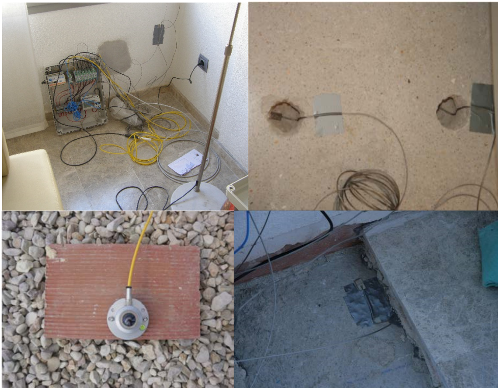
Figure 6: Data logger and sensors in the basement. Pyranometer on the roof.
