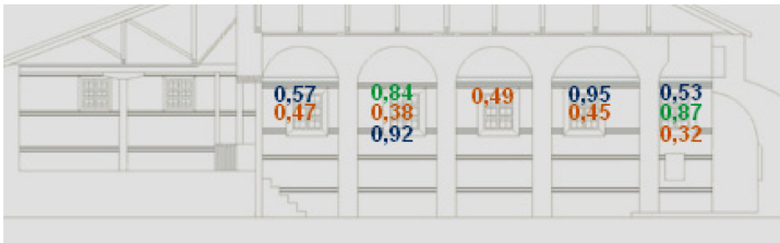
Figure 13: Internal colonnade. Regions with small values of the strength / demand R_M out-of-plane tensile behaviour (orange color), R_r in-plane shear behaviour (green color), R_\sigma in-plane tensile behaviour (blue color).
