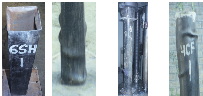
Figure 1: Photographs showing failure modes and test setup of columns.
